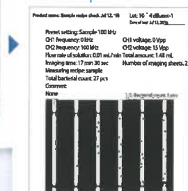
Measured data and photographs are recorded together with setting conditions and output in a PDF format
