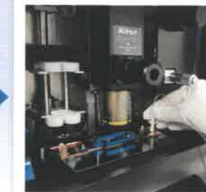
Connect the waste tube to the waste port on the ELESTA™ chip
